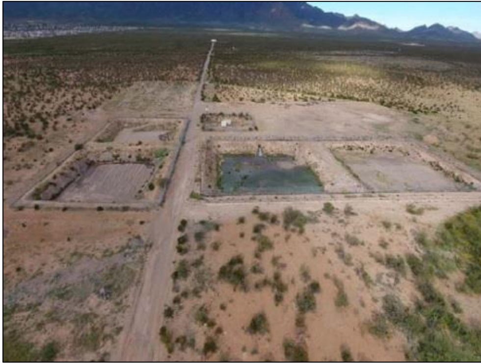
Figure A-7: Infiltration basins
